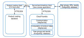
Fig. 1: Block Diagram of the Prototype's Architecture
