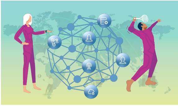
Fig. 1. Example highlighting the TaHiL enabled Internet of Skills: Human skills are digitized and transported over intelligent networks, before being applied via actuators, robots, or other means. The tactile information control loop in the Tactile Internet limits the real-time loop latency to 1 ms.
